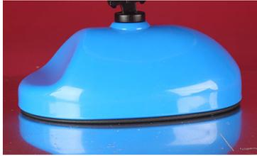
If ear-muffs with fluid filled cushions are under test, then resistance to leakage must be assessed. A vertical load of  $28 \pm 1$  Newtons is applied to the cushion for 15 minutes and any leakage caused will constitute a test failure.
