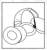
Change the cushions (foam), place it correctly on the earmuffs. Make sure they are aligned correctly.
