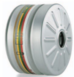
Dräger X-plore® Rd40 filter (according to EN standard): 620 A2B2E2K2 Hg P3 R D
