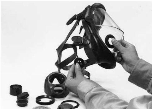
FIGURE 19 Removing the Inhalation Connector
