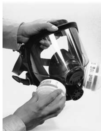
FIGURE 3 Attaching Air-Purifying Elements
