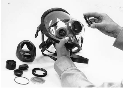
FIGURE 17 Removing the Speech Diaphragm Housing on the 7600 Series
